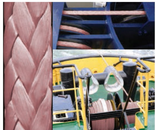
As a steel wire replacement Donaghys winchline is lighter, safer and stronger - for mining applications, industries and marine.
